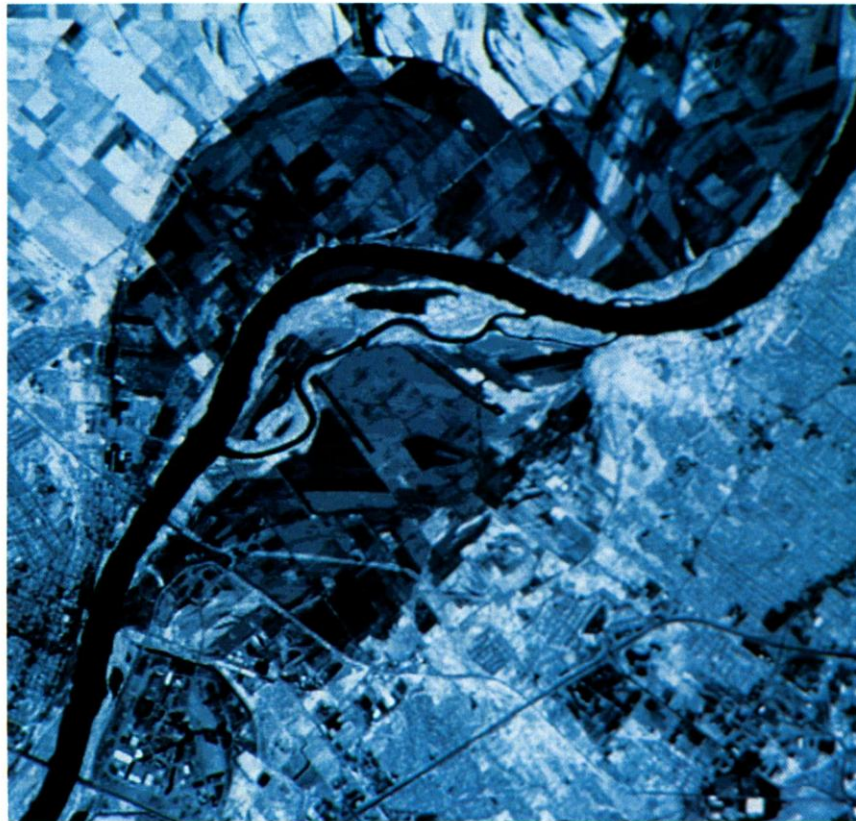
Figure 5 Mathematical approach image by adding together TM band 4 (1988), TM band 4 (1993), and TM band 7 (1993).
